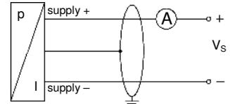
3-wire-system (voltage, ratiometric)
