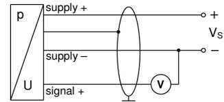
**⚠** For the electrical connection, a shielded and twisted multicore cable has to be used.
